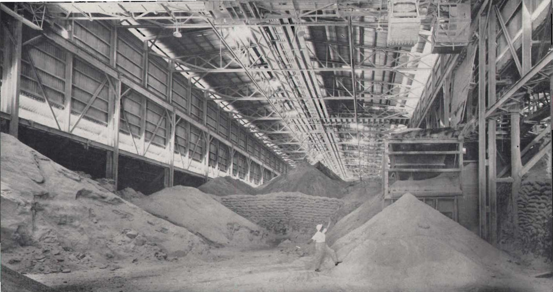
Australian farmers used about 2½ million tons of superphosphate in 1960-61, spending £20 million on topdressing alone. This giant fertilizer storage shed in Melbourne has a capacity of 3,000 tons. Both superphosphate and mixed fertilizers are stored here for up to a month until they have matured.
